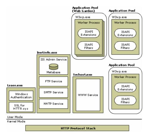
Figure-1: Architecture of IIS 6.0 (source: Microsoft Technet)
